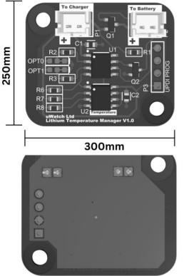
Prevents solar panel from charging battery below 1C. Prevents damage to lithium battery. Periodic checks reduce battery consumption. Installed between rechargeable battery, and solar controller.
